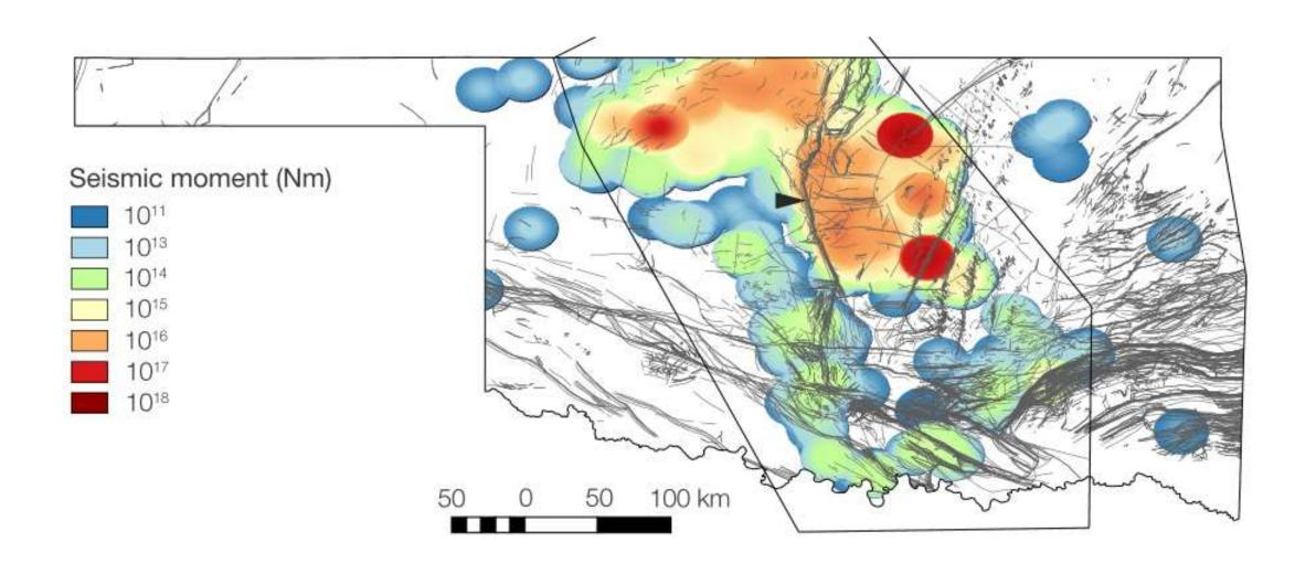
Total seismic moment release in Oklahoma
