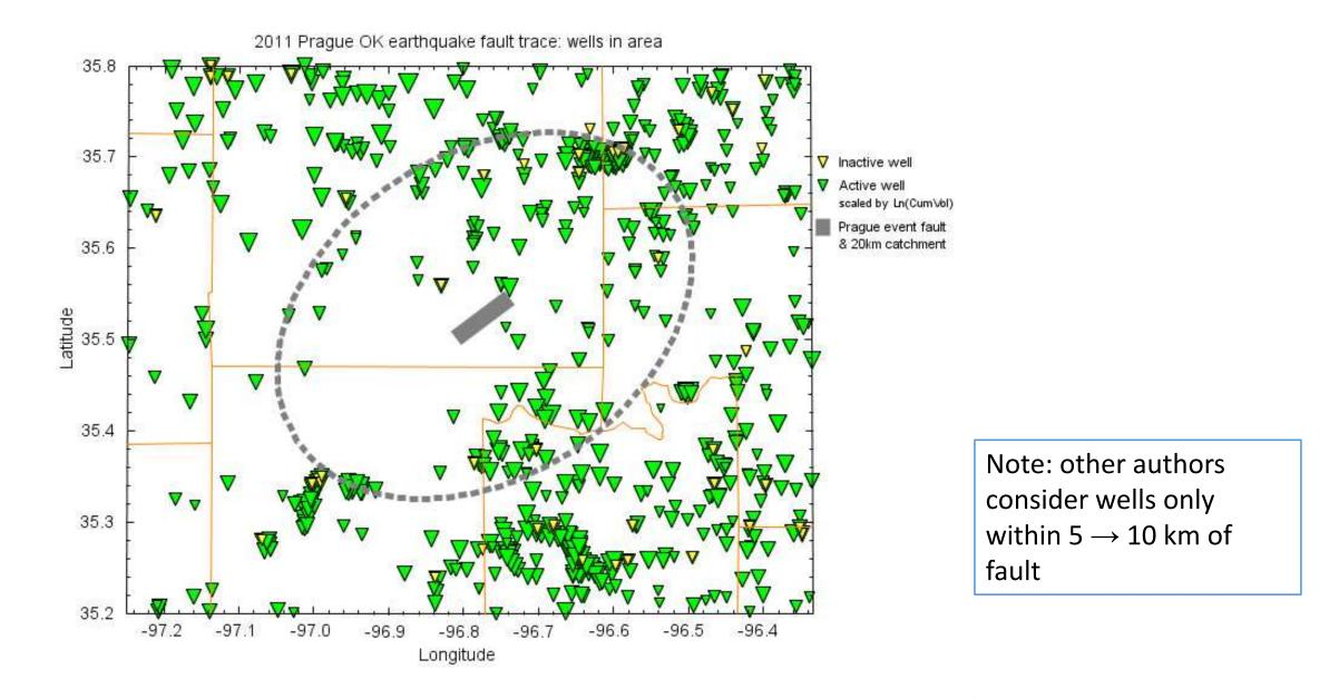
Attribution: active and inactive wells near 2011 Prague OK earthquake fault
