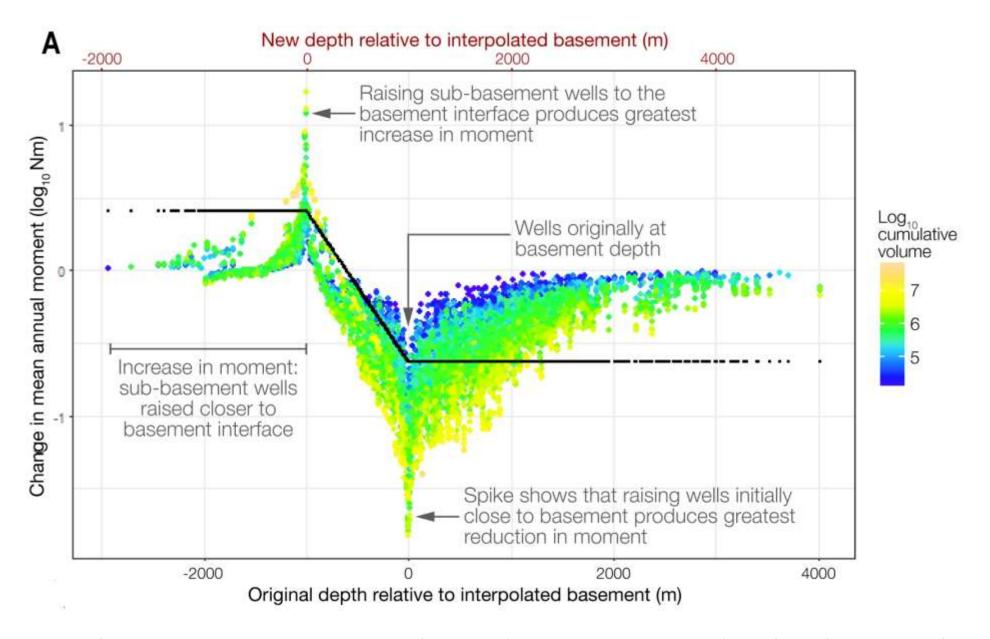
BN inferences about seismic moment release due to injection depth relative to basement, not captured by ordinary linear regression (black dots)
