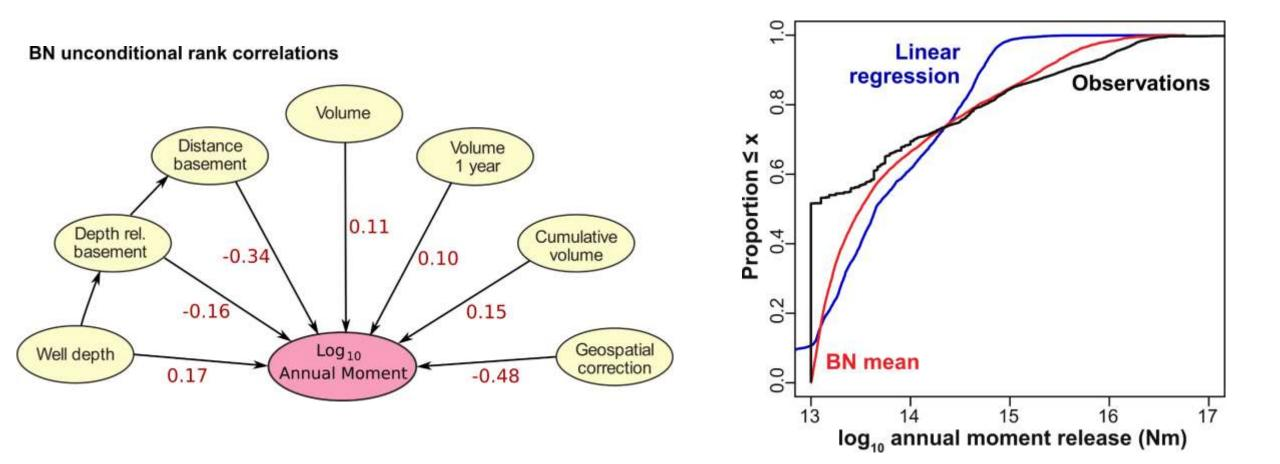
Induced seismicity Bayes Net: correlating seismic moment with well parameters (left), and superior performance relative to traditional regression analysis (right)
